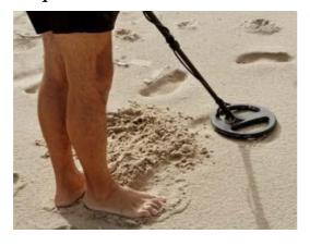
The first thing to check is that you have the head, where the coil is, as close to the soil surface as you safely can.
