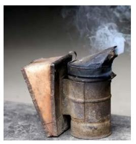
These come in various styles. There is a cylinder with a section at the bottom where the material you burn is placed and a nozzle at the top to direct the smoke.
